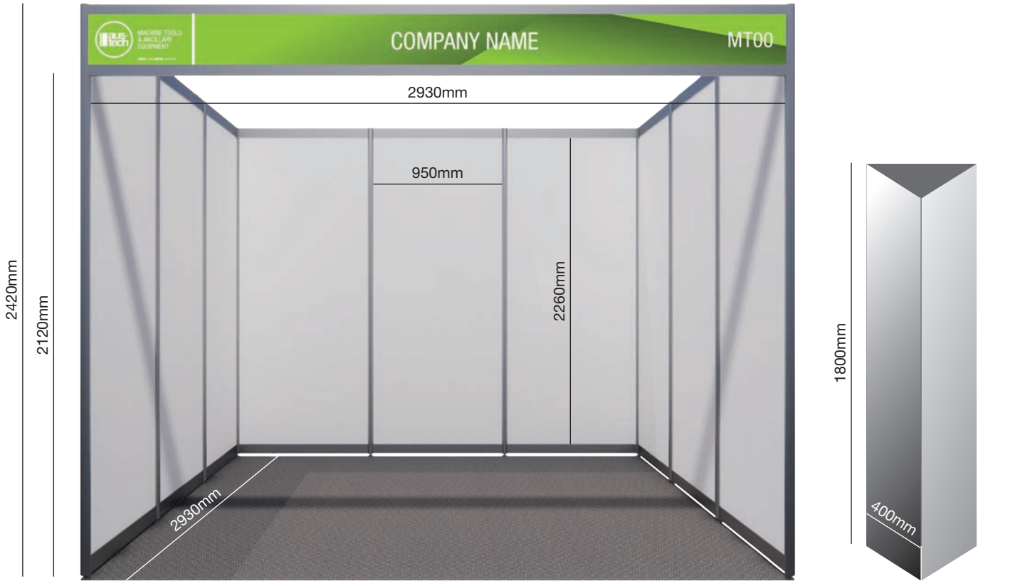
Shell Scheme Signage Option 1 – Fascia: all posts protrude 20mm into the stand
